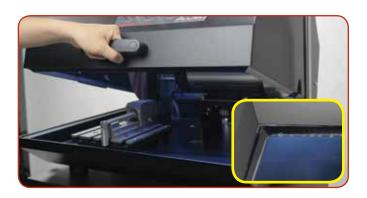
The cover has a large, shatterproof viewing window for operator safety, and an angled internal edge that eliminates external dripping. A safety switch quickly stops blade rotation if the cover is raised during operation.
