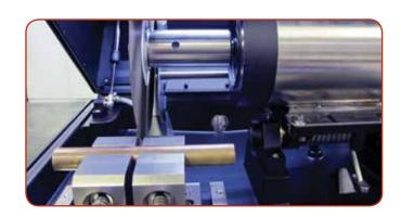
Extra-long 5" (127 mm) distance between the blade and motor allows longer/larger parts to be sectioned.
