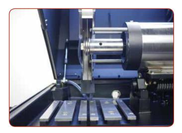
Two T-slot tables allow the use of a wide range of clamping and fixturing options available to accommodate a variety of sample shapes and sizes.
