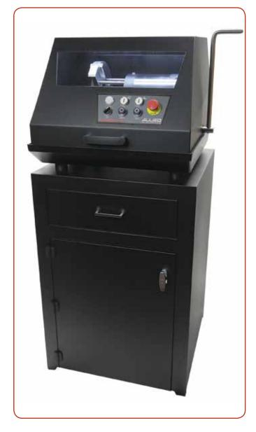
The cabinet/stand is designed to provide a solid platform to support the PowerCut 10x™. Made of cross-braced aluminum for vibration control, strength and stability, it is configured for proper routing of electrical cords, drain hose and coolant supply tubing. It features a large, deep drawer for storing fixtures, tools and blades, and a hinged door to house the recirculating coolant system. One (1) #5-4210 Roller Cart is included.
