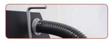
The extraction port is used to remove smoke and odor from the cutting chamber. The 3" diameter port allows a hose to connect with stand-alone or facility filtration systems.
