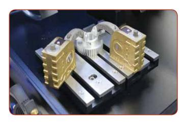
The vertical adjusting clamp can be positioned in any orientation throughout the T-slots in the tables. The height adjustable lever allows various size samples up to 2.25" (57 mm) thick to be secured. Interchangeable pads are available for a variety of sample shapes. Each clamp includes one (1) angled pad and one (1) flat pad.
