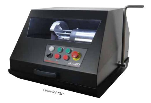
The **PowerCut 10x™** is a powerful, reliable cut-off saw designed for low to high volume applications. It accommodates blades up to 10" (250 mm) in diameter, allowing a wide variety of sample shapes and sizes up to 3.75" (95 mm) thick to be sectioned.
