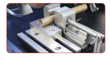
This platform has a height equal to the base of the vise, allowing the unclamped portion of the sample to be supported during the sectioning process. It prevents this portion from falling as the end of the cut nears, minimizing the burr upon completion. It can be positioned anywhere along the T-slots.
