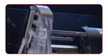
Dual coolant manifolds with directional jets provide uniform blade/sample lubrication.
