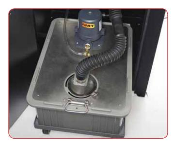
The 7-gallon (26.5 L) recirculating coolant system is constructed of corrosion resistant materials for maximum durability. The reservoir fits conveniently in the available cabinet, or can be placed near the machine in existing lab furniture. A removable catch screen enables quick cleaning of larger particles. Baffles inside the reservoir trap particulates. The optional roller cart (included with cabinet) allows easy transfer for cleaning.
