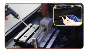
After sectioning, simply adjust the valve to redirect coolant from the blade to the cleaning hose.
