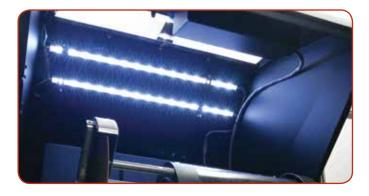
LED illumination inside the cover allows easy observation of the sectioning process through the large viewing window.
