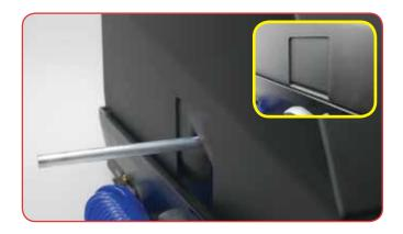
The side plate in the cover can be removed for convenient cutting of long samples such as bar stock.
